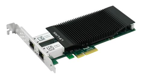
LRES2002PT-POE is a PCIe x4 PoE 1G dual-port copper industrial ethernet network adapter based on the Intel I350 chipset, be developed independently by Shenzhen Lianrui Electronics Co., Ltd and is compatible with x8, x16 lanes. The PoE adapter is designed mainly used on industrial field vision inspection server and equipment, vision field client, fast moving Ethernet data transmission equipment etc. It's also suitable for ordinary servers.
